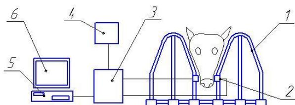
1 - separation grid; 2 - photoresistors; 3 - pulse accumulator; 4 - counter; 5 - system unit; 6 – monitor
