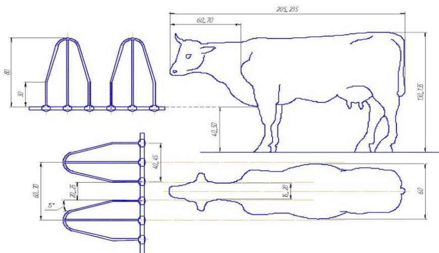
Figure 3: Dimensions of the separation grid
