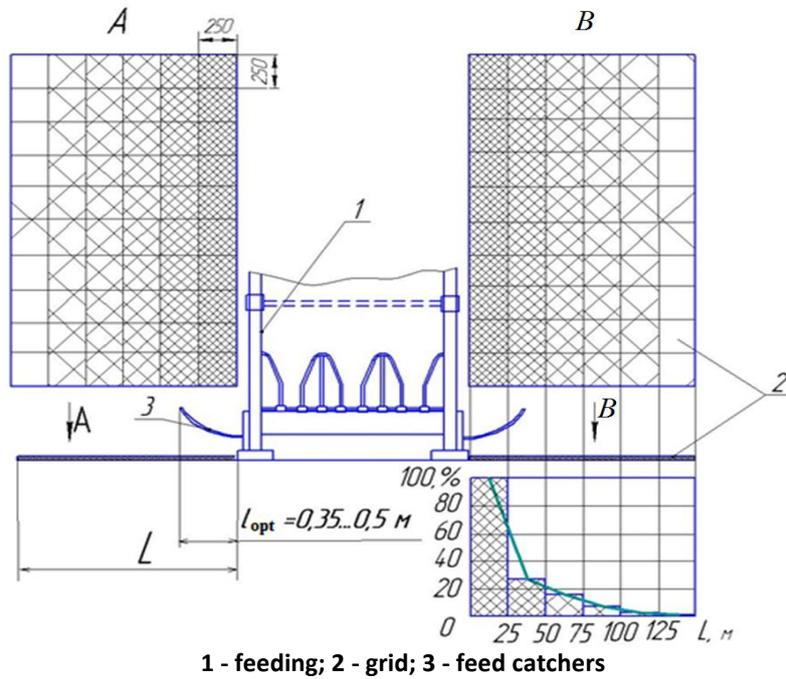
Figure 4: Distribution of feed loss (%) depending on the distance from the edge of the self-feeder
